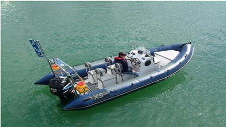
At this sort of size the "serious end" of ribbing will also have double side by side consoles, and multiple seating. What you get in a craft like the XS 600 shown here are typically Deeper V hulls and higher bows than the leisure craft.
